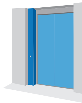
Location of the Maintenance Access Panel
